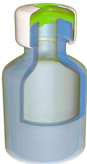
Volume render of a glass vial with rubber seal and aluminum cap SKYSCAN 1275 – Voxel size 10 \mu\text{m}
