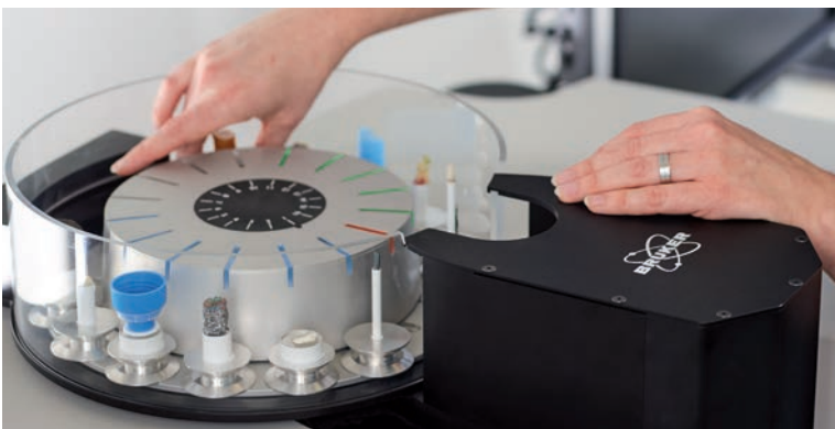
Change samples at any time without interrupting an ongoing scan
