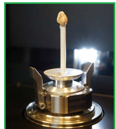
For highest resolution rely on the integrated micro positioning stage and insert the sample manually
